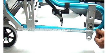
pic. 18: Displacement of the wheels plate
