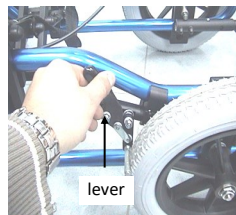
pic. 5: Activating the brake lever
