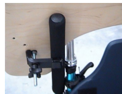
pic. 26: tubular armrest mounting
